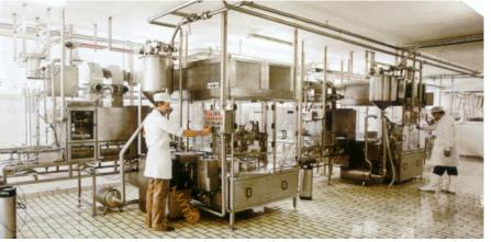
and on pipelines, use an aqueous solution (preferably hot) with 30% of the product (300 grm/litre). Rinse accurately at the end of the work.
