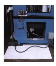
**NB.** The absorbency of **DESORB 7302** varies considerably depending on the viscosity of the oil. As can be seen from the graph, with low viscosity oil, ISO 22, an amount of oil equal to 50% of the weight of the towel can be absorbed. With denser oils this value increases up to 75% times.
