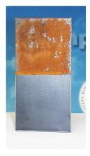
tects the metal like a paint, but can easily be removed before the use of the piece treated.
